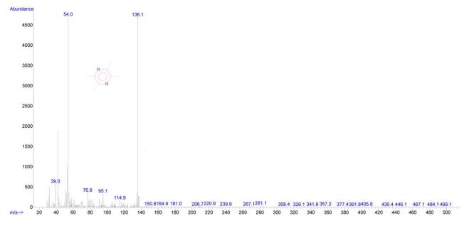
Fig. 11. Mass spectrum of tetramethyl pyrazine in ancient *Ephedra* extract. [Color figure can be viewed in the online issue, which is available at wileyonlinelibrary.com.]
